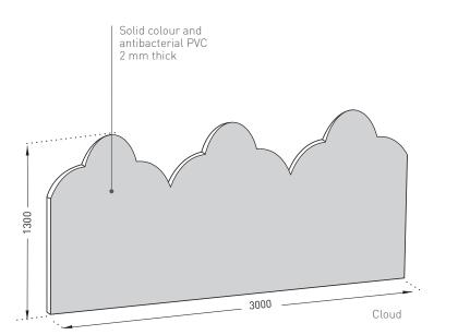
• Description: protection and covering decorative fresco (Cloud or Wave Decofresc as manufactured by SPM) from rigid and antibacterial PVC achieving Bs2d0 reaction to fire classification with solid colour and slightly textured and matte surface ("Hydr'X" finish as manufactured by SPM). 3 m long, 1.30 m high (indivisible), 2 mm thick.
